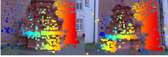
Figure 3. Putative matches obtained with the classical SIFT algorithm, which seeks matches over the entire image. The figure shows images 7 and 3 from the Fountain dataset. Corresponding points are marked by points of the same color and size with color varying with position along the X -axis in the left image and size varying with position along the Y -axis.
