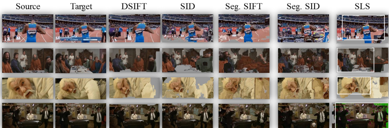
Fig. 8. Dense flow with scene motion. Image pairs presenting different scale changes in different parts of the scene, due to camera and scene motion. Correspondences from Source to Target images estimated using [9], comparing DSIFT [8], SID [19], Segmented SID and segmented SIFT, both from [37] and our SLS, shown here with the automatically determined crop region in white (Sec. 3.5).
