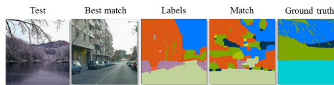
Fig. 11: Failed semantic segmentation result. A typical error due mostly to poor selections of reference images. The impact of reference selection on segmentation accuracy has been noted in the past by others (e.g., [14]).
